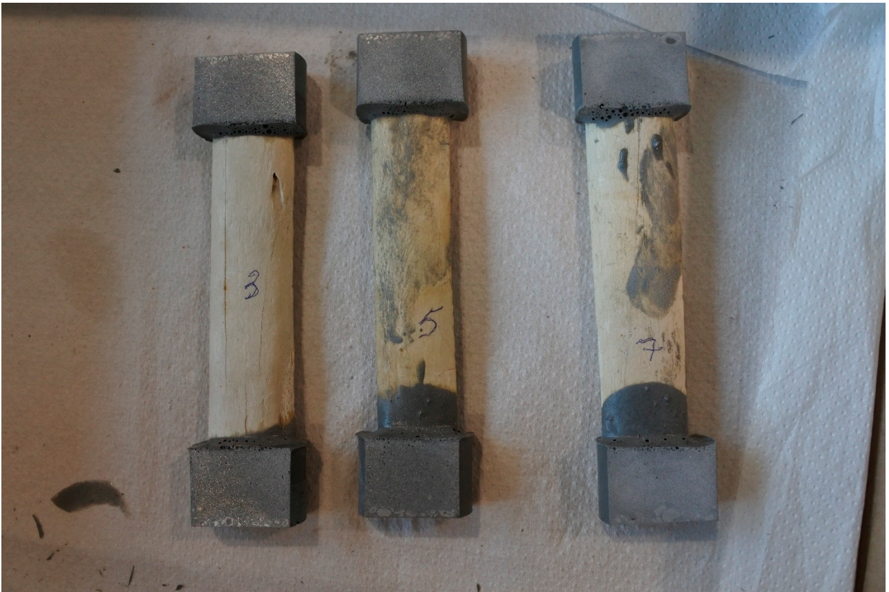
Figure S1: Tibia dried samples. Dried samples ready for uniaxial tensile test.
