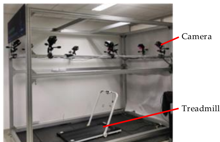
Figure 4. The NOKOV optical three-dimensional motion capture system.
