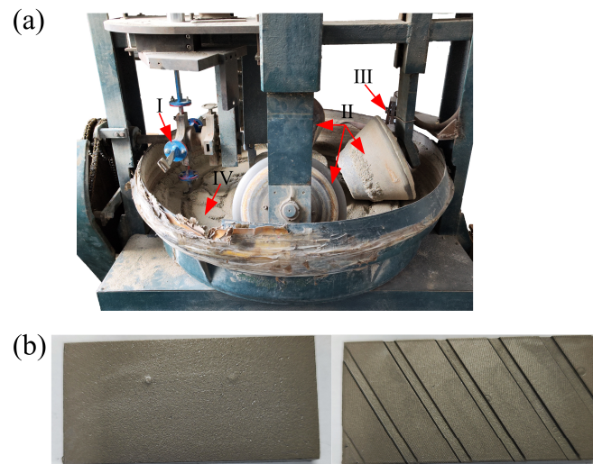
Figure 5. (a) JMM abrasive wear tester: (I) Sample holder, (II) Suppression roller, (III) Soil scraper, (IV) Rotary abrasive bin; (b) Samples of CS and BRS.
