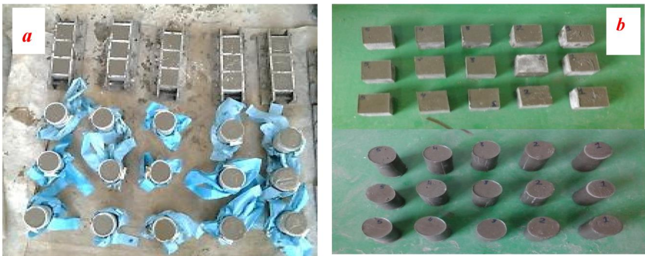
Figure 3. Preparation of specimens for mechanical properties tests: (a) PRG in molds; (b) PRG cubes and cylinders.
