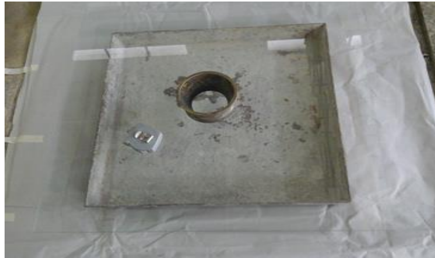
Figure 4. Test setup for flowability test.
