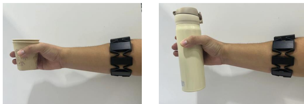
Figure 2. Collecting sEMG signals while grasping different objects with human hand.
