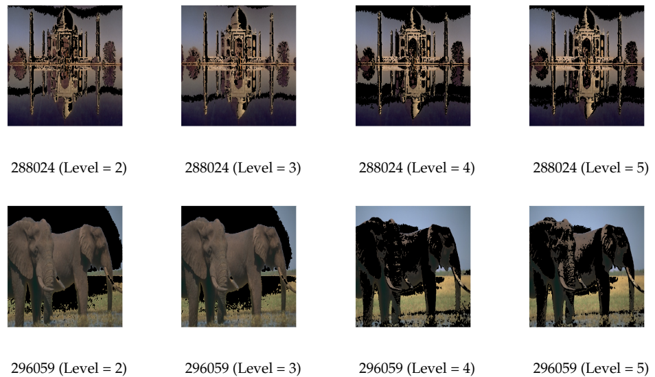
Figure 12. Results of thresholded images with different thresholding levels of MGWO based on the Otsu method.
