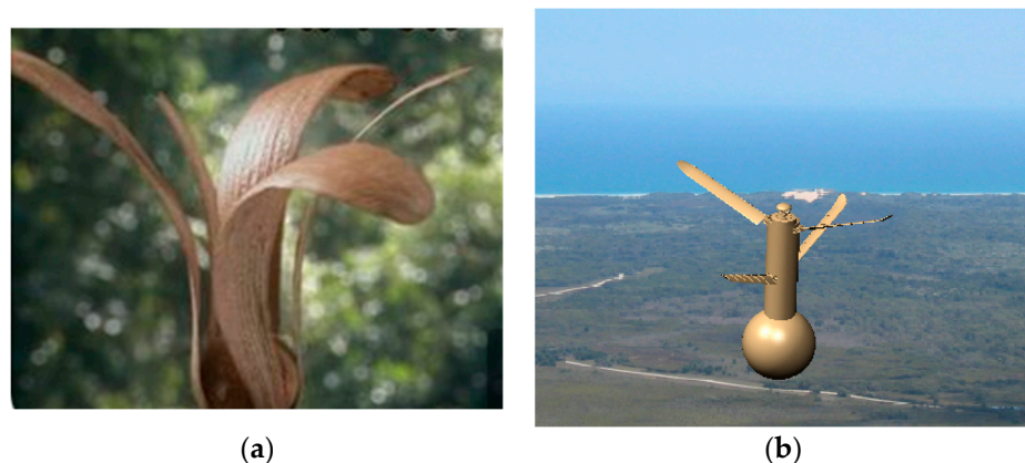
Figure 2. Design modeling sketch of the initiated flyby configuration. (a) Instantaneous morphology of Chinese parasol seed shedding; (b) initiated flyby configuration.
