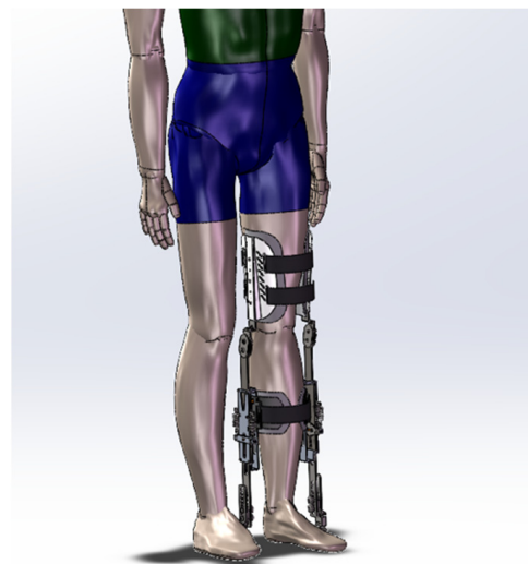
Figure 8. Exoskeleton diagram of the knee joint.
