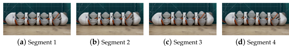
Figure 24. Steps of peristaltic motion contractions shown on the PALAM robot (see Figure 25 for elongated state).
