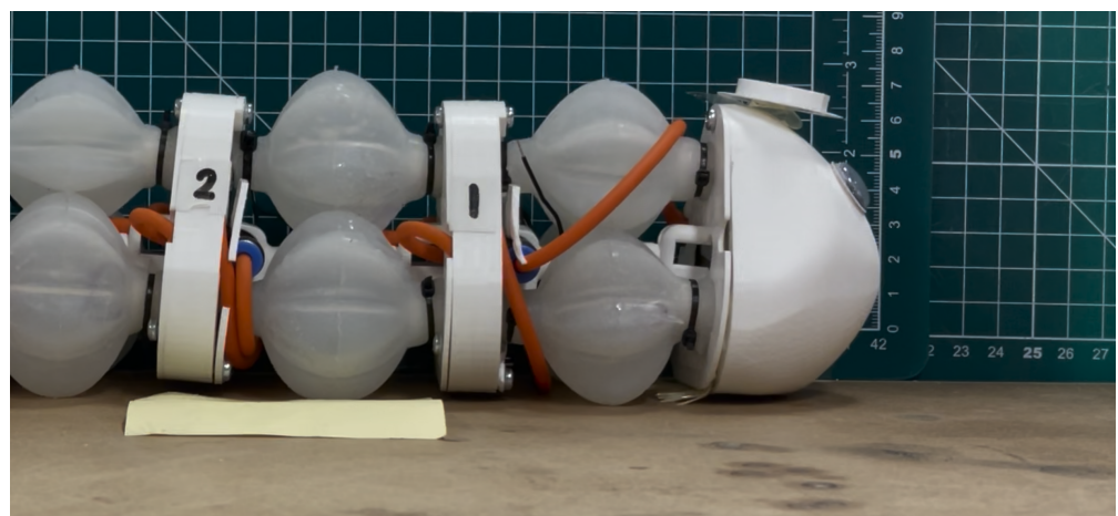
Figure A15. Photo of setae (bristles) added to the head of the worm.
