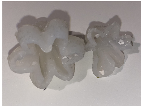
Figure A13. Photo of one of the ruptured PAMs. The rupture happened in about one quarter of the PAM during the demoulding process. Small remnants of the inner mould are visible.
