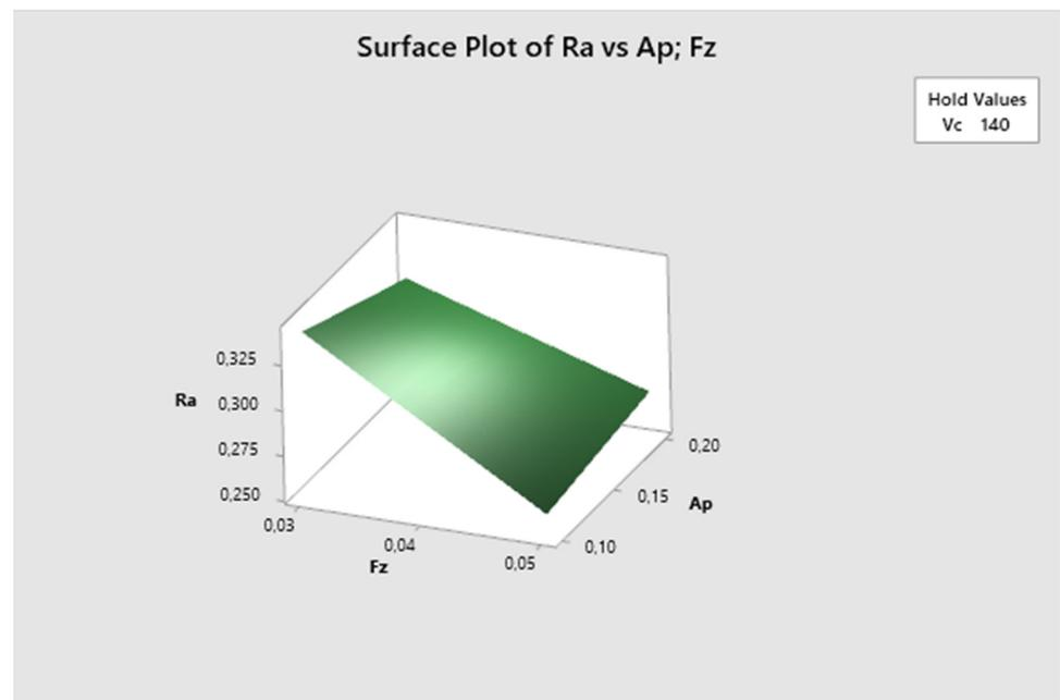
**Figure 12.** The first experiment—surface plot of  $Ra$ — $a_p$ ;  $f_z$ .
