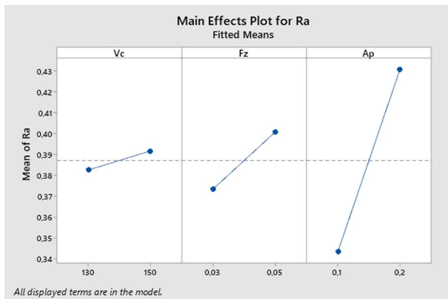
Figure 26. The third experiment-main effects plot for Ra.
