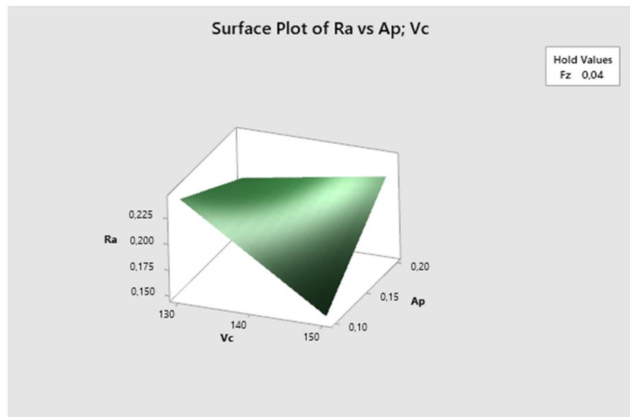
Figure 20. The second experiment-surface plot of  $R_a$ — $a_p$ ;  $v_c$ .
