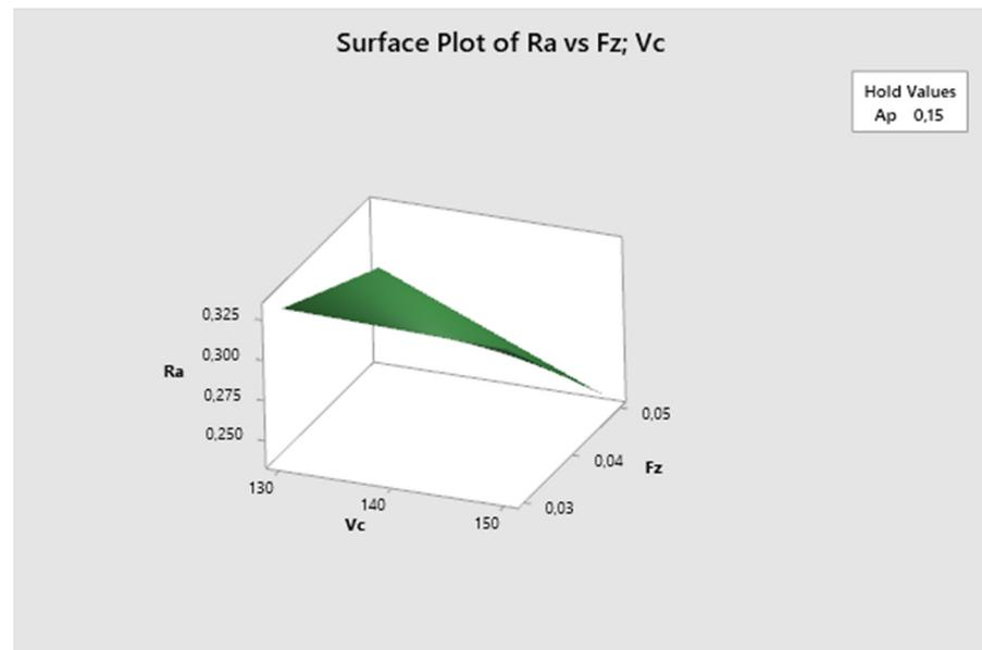
**Figure 10.** The first experiment-surface plot of Ra— $f_z$ ;  $v_c$ .
