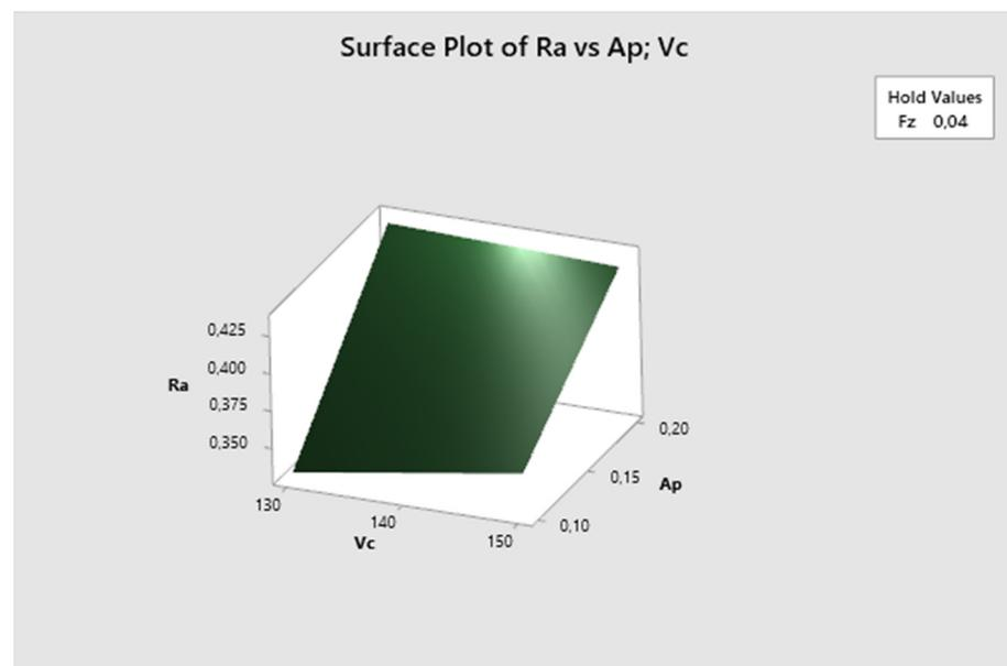
Figure 29. The third experiment-surface plot of  $R_a$ — $a_p$ ;  $v_c$ .
