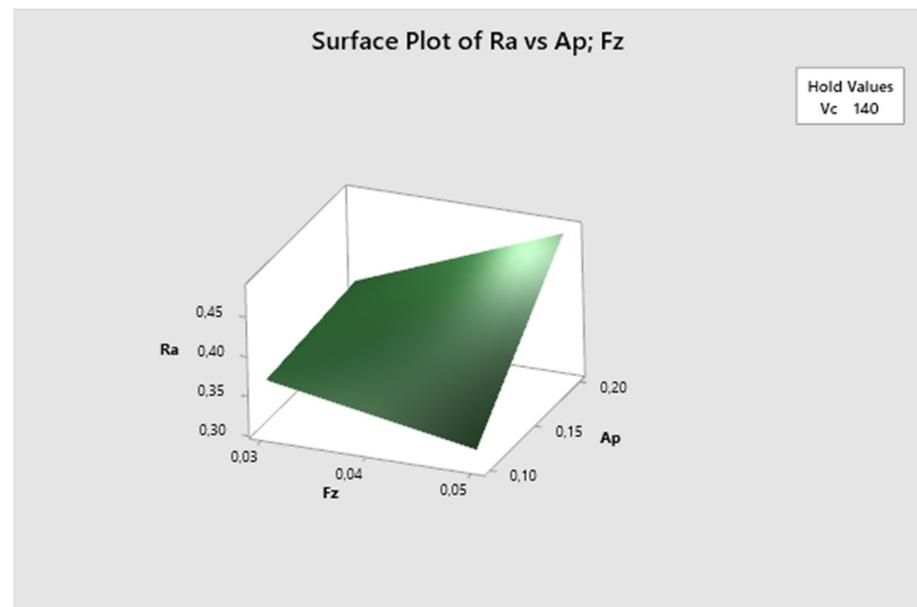
**Figure 30.** The third experiment-surface plot of Ra— $a_p$ ;  $f_z$ .
