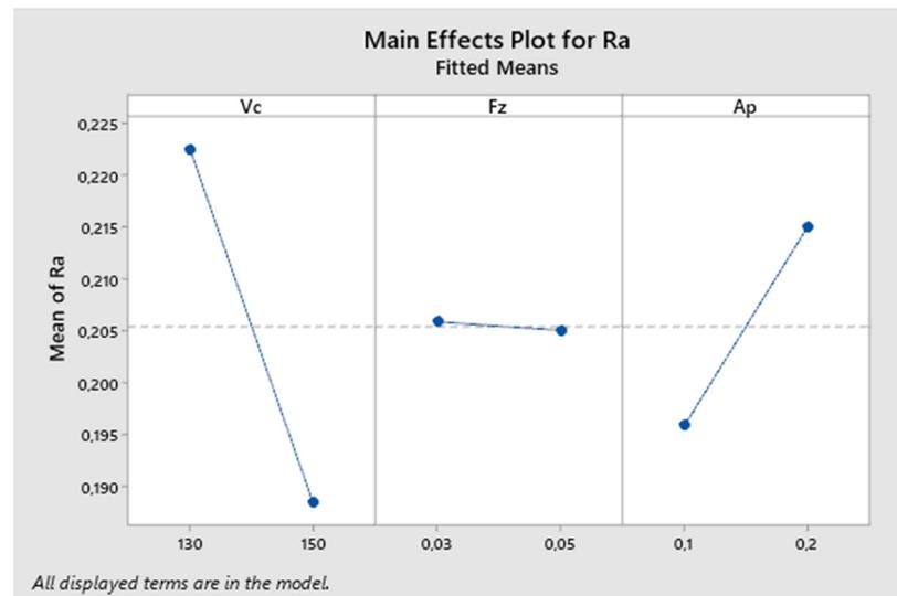
Figure 17. The second experiment-main effects plot for Ra.
