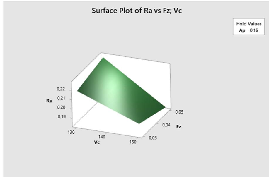
Figure 19. The second experiment-surface plot of  $R_a$ — $f_z$ ;  $v_c$ .
