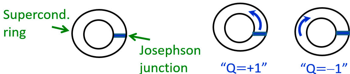
Figure 4. A “flux qubit”, the system used in ref. [20] for a test of MR (idealized).
