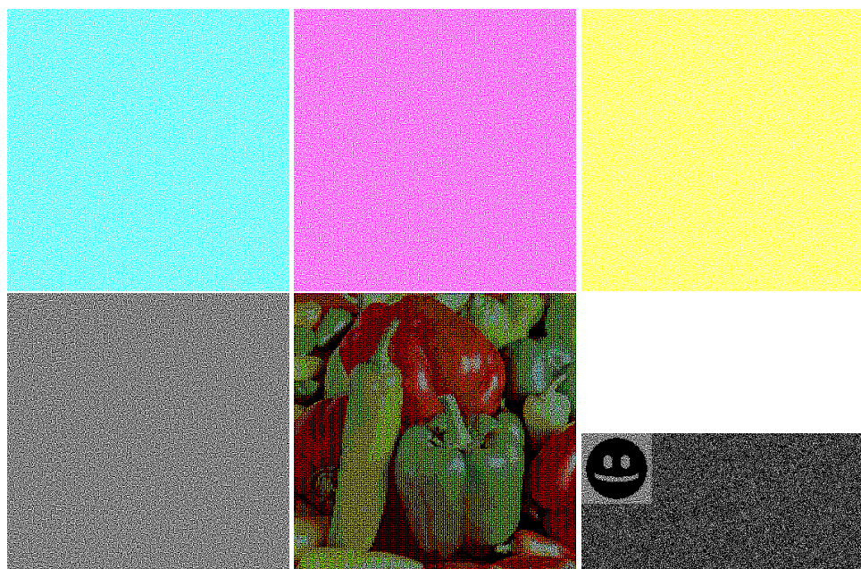
Figure 7. Fold method in color visual cryptography: C, M, Y color shares, a mask, stacking result and revealed secret binary image.
