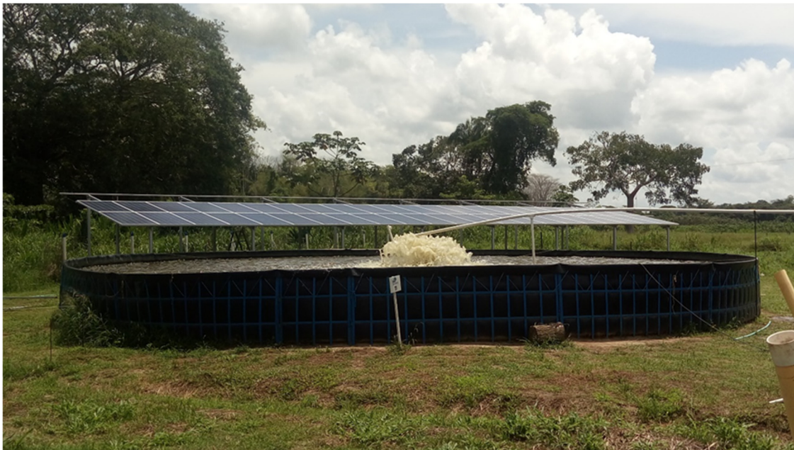
Figure 1. Image of the production system, high-density polyethylene (HDPE) geomembrane tanks, and photovoltaic system.
