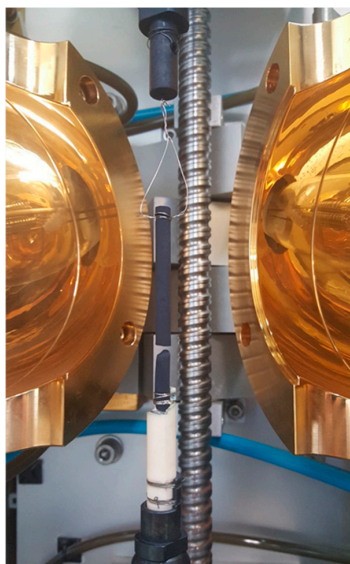
Figure 2. Photo of a polycrystalline feed rod and seed ready for the floating-zone growth. They are placed at the center of the two elliptical mirrors of the infrared mirror furnace at Kyoto. In this example, a polycrystalline seed is used, rather than a single crystal.
