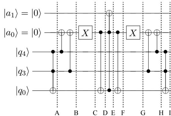
**Figure 6.** The reversible circuit over Toffoli gates and CNOTs, with two ancillae, for labelling the states 000 ↔ 111.
