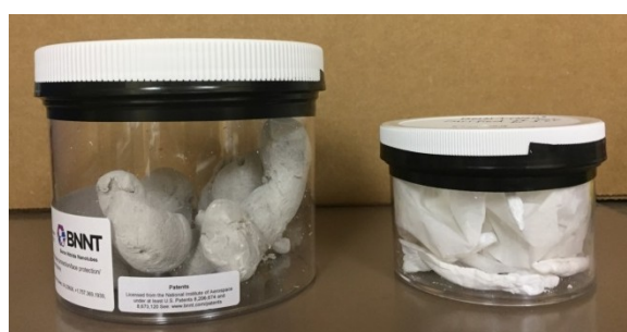
Figure 18. Photograph of 500-mg sample of as-received BNNT (left) and 500-mg sample of BNNT following purification at the National Institute of Aerospace (NIA) at 600\text{ }^\circ\text{C} for 1 h (right).
