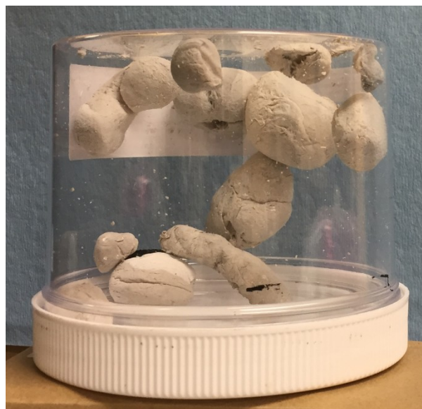
Figure 2. Photograph of 500-mg sample of bulk boron nitride nanotube (BNNT) material from BNNT, LLC, supplier.
