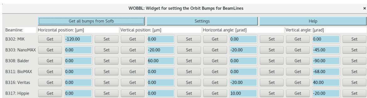
**Figure 9.** Widget for setting the Orbit Bumps for BeamLines (WOBBL) interface containing the beamlines which are in normal operation for the 3 GeV ring and also the Multipole Injection Kicker (MIK). The widget has input fields for setting each of the four types of bump changes, for each beamline.
