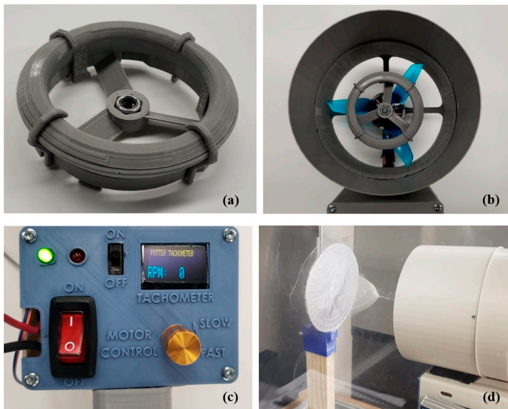
Figure 8. (a) Spinneret assembly and fan blade mounted on motor shaft, (b) 3D-printed spinneret assembly, (c) control panel, and (d) fiber mat spun with HD.
