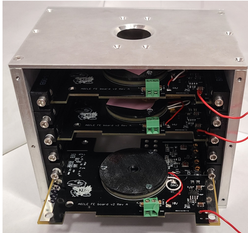
Figure 4. A photograph of the CubeSat mock-up used in the laboratory tests.
