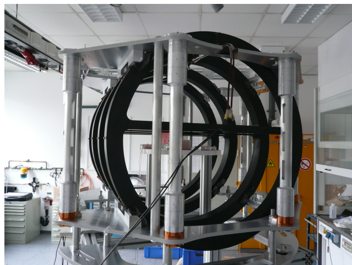
Figure 3. Fully assembled magnet system in the laboratory.
