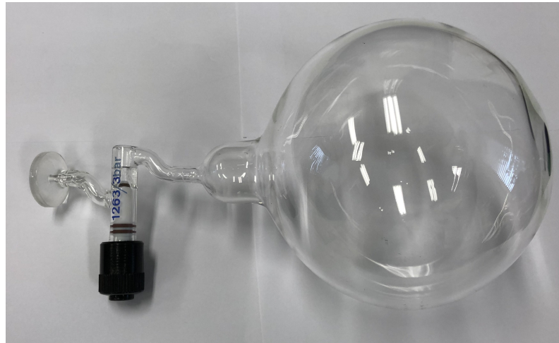
Figure 4. Glass ball, manufactured at FZ Jülich, for the storage of polarized ^3\text{He} .
