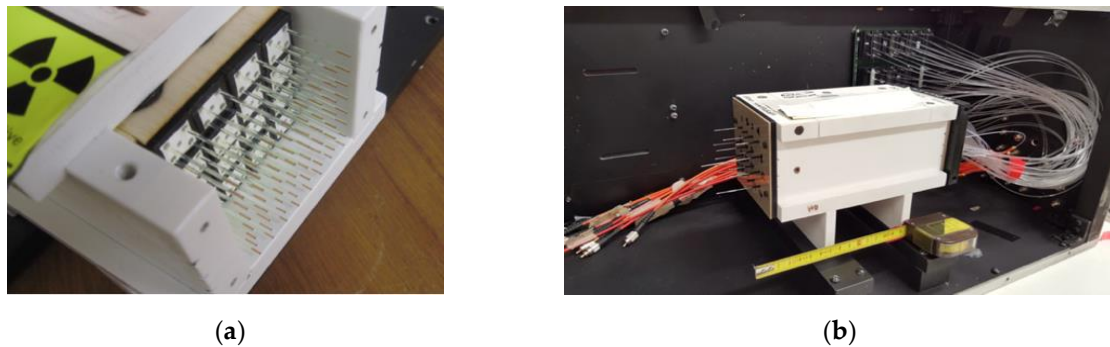
Figure 3. (a) The 4 \times 4 modular array during assembly. (b) Fiber optic waveguides used to transmit the WLS light to SiPM photosensors positioned outside of the beam region for this specific test. In the picture, the incoming electron beam is incident from the left on the 4 \times 4 modular array enclosed within the white mechanical housing.
