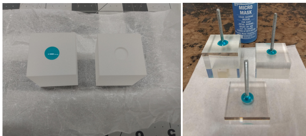
Figure 2. Ground (left) and polished (right) SF57HHT glass tiles of various dimensions.
