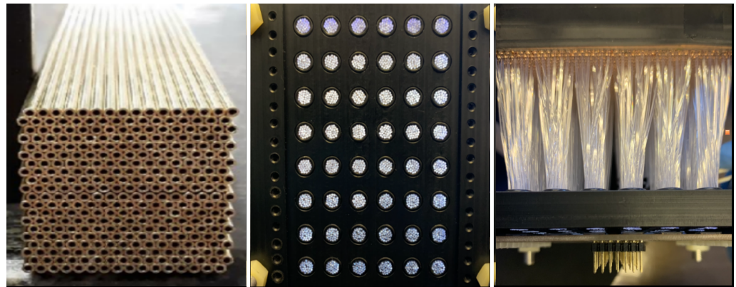
Figure 1. FoCal-H 2021 prototype module with 1440 Cu tubes ( left ), grouped scintillating fibers at the back of the detector ( center ) and 16 (out of 48) mounted Onsemi MICROFC-60035-SMT-TR1 SiPMs at the back of the detector ( right ).
