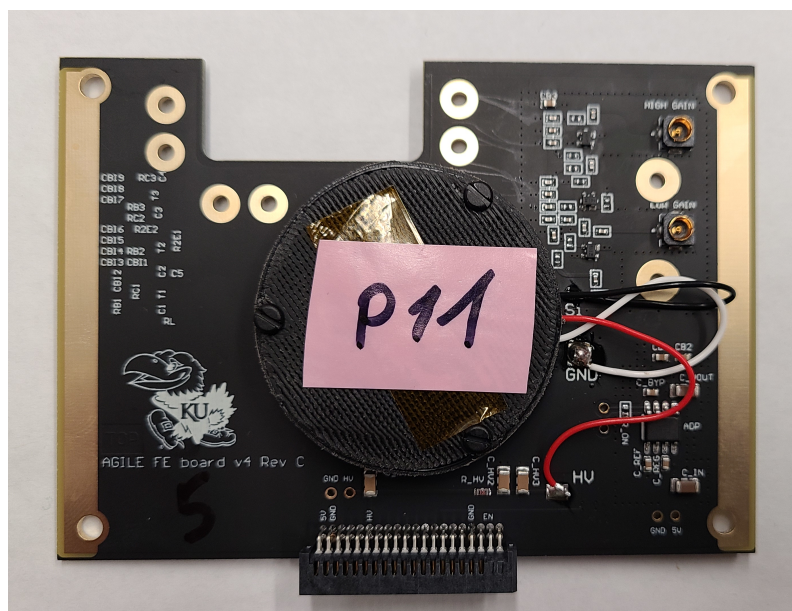
Figure 3. Photo of one layer of the silicon detector (300 \mu\text{m} thick and 20 mm diameter) in its protective case and its readout electronics to be sent into space in collaboration with NASA (AGILE project). The silicon is used as an absorber to detect and measure the different particles emitted in cosmic rays.
