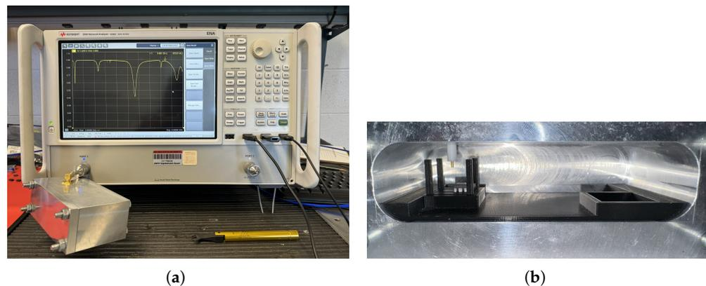
**Figure 2.** (a) Experimental setup with resonant cavity connected to the VNA. (b) IC placed on a plastic platform and holder inside the resonant cavity.
