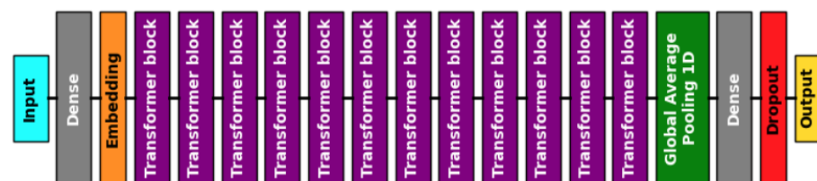
Figure 4. Architecture of the designed BERT for the DA regressor.
