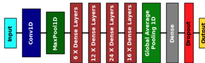
Figure 5. Architecture of the designed DenseNet-121 for the DA regressor.
