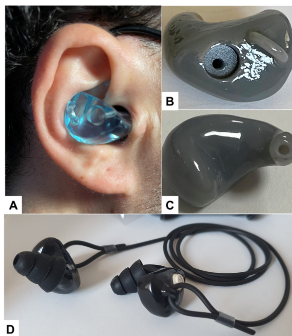
Figure 1. (A): Dynamic earplug worn by a subject; (B): anterior view of the dynamic earplug; (C): posterior view of the dynamic earplug (without ear tip); (D): dynamic earplugs with ear tips.
