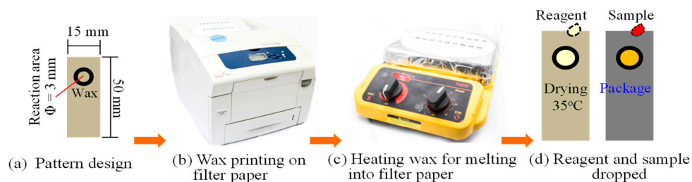
Figure 1. Schematic illustration showing main steps in fabrication procedure for paper-based chip.
