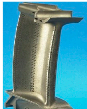
Figure 2. The turbine blade surface with film cooling holes [6].
