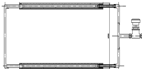
Figure 11. Flat loop thermosiphon made from a polymer composite [41].
