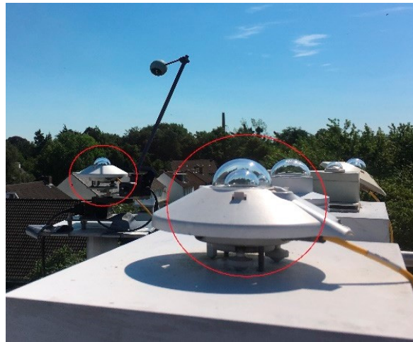
Figure 1. Photo of a pyranometer [6].
