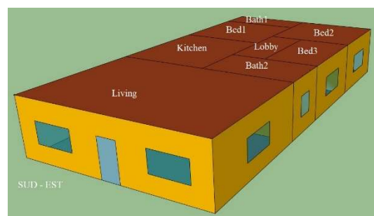
Figure 4. Thermal zones of the simulated building.
