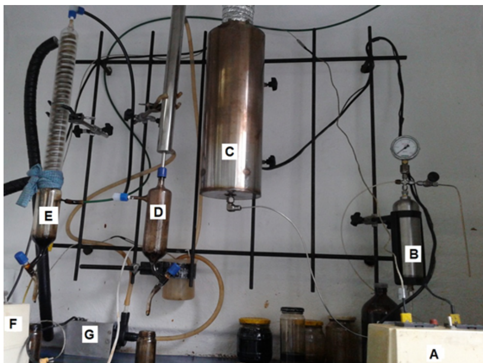
Figure 1. Pyrolysis system: (A) Heat or temperature controller; (B) Pressure maintainer; (C) Main electric furnace (biomass); (D) Condenser with 100 °C; (E) Condenser with 5 °C; (F) Cooler; (G) Hot water pump.
