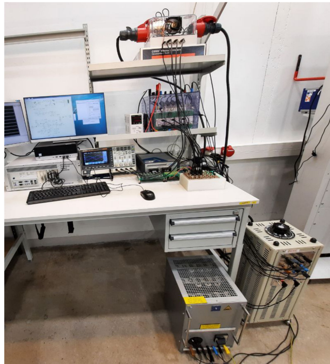
Figure 6. The setup for the current transducers box and the loading test of the inverter.
