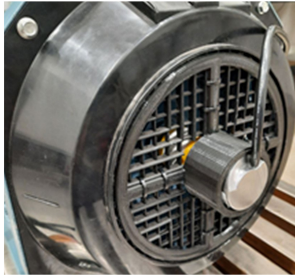
Figure 4. The 3D printed holder and coupling for mounting the encoder on the motor.
