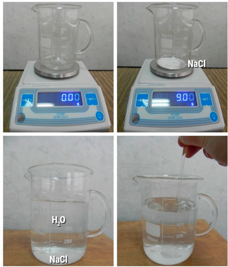
Figure 4. The process of preparing a model seawater solution.
