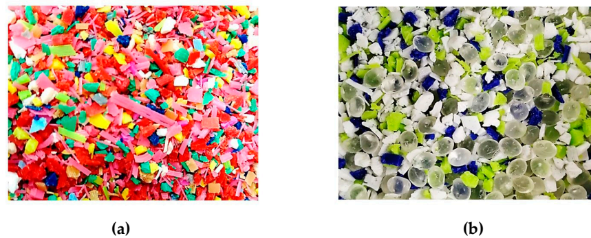
Figure 5. Recycled PLA waste. (a) 100% shredded PLA, (b) combination of recycled (70%) and virgin PLA pellets (30%).
