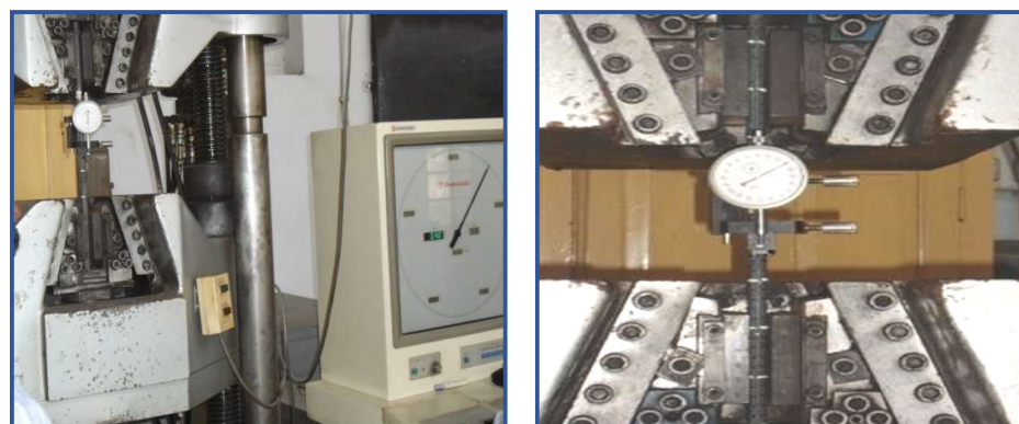
Figure 3. Steel bar tension test in progress using digital UTM (ASTM A-370-03).
