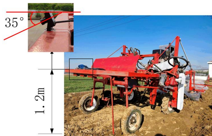
Figure 1. The structure of cuttage and film covering multi-functional machine for low tunnels.
