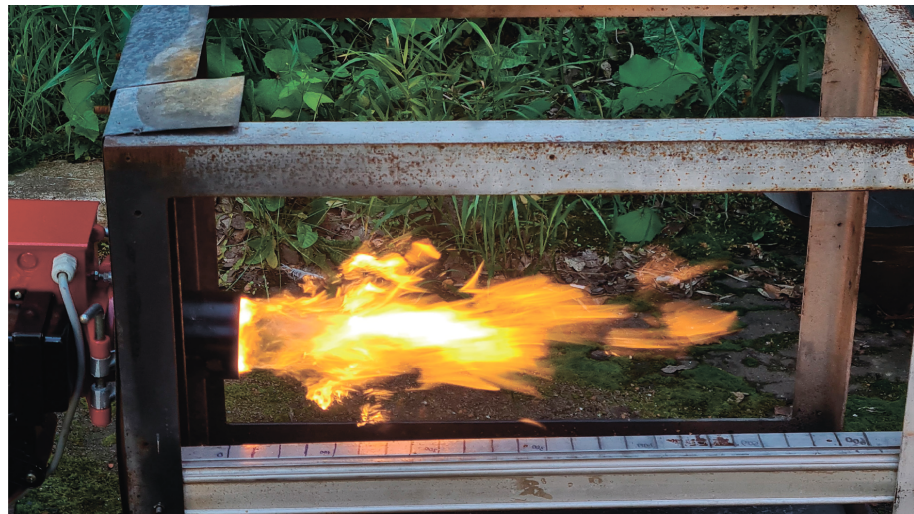
Figure 11. Diesel fuel combustion in OILON burner.
