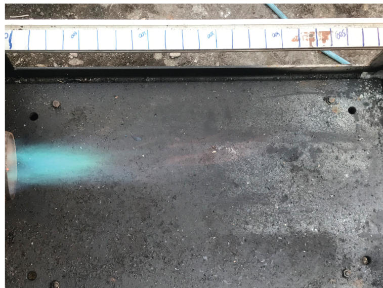
Figure 9. Propane combustion in OILON burner.
