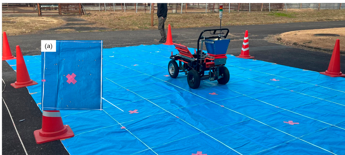
Figure 16. Grid arrangement and data collection: (a) 65 cm × 65 cm grid seed distribution.
