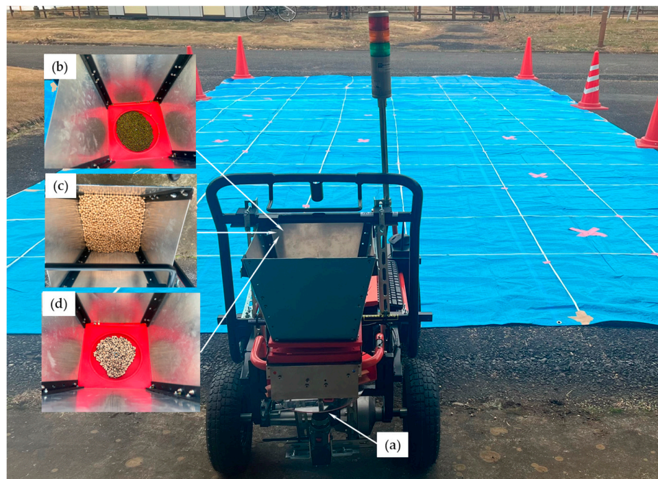
Figure 11. Evaluation of the seeding mechanism and autonomous vehicle: (a) spreading disk; (b) mung bean; (c) cowpea; (d) chickpea.
