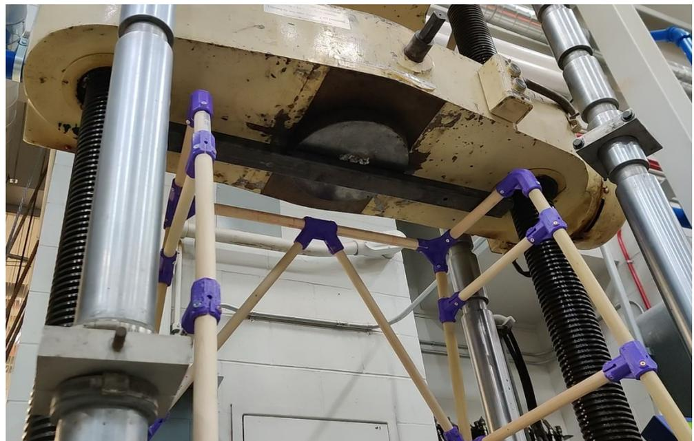
**Figure 5.** Testing distributed load that replicates the span of a fists on the walker.
