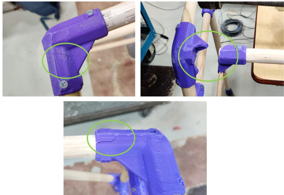
**Figure 11.** Sample images of failure occurring at the 3D-printed Ang 3 Connector part after horizontal walker testing.
