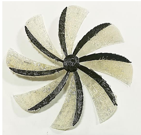
Figure 7. Additively manufactured multi-material propeller blade.
