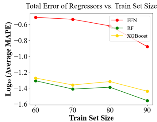
Figure 9. Impact of train set size on the overall performance of three regressors in the estimation of process parameters. The overall error is shown by the log 10 (MAPE) metric.
