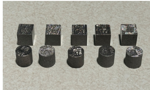
Figure 2. Printed cubical and cylindrical parts.
