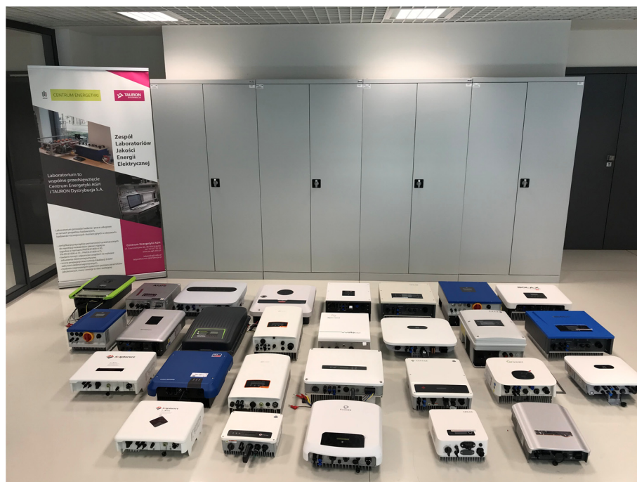
Figure 9. Collective photo of the tested PV inverters.
