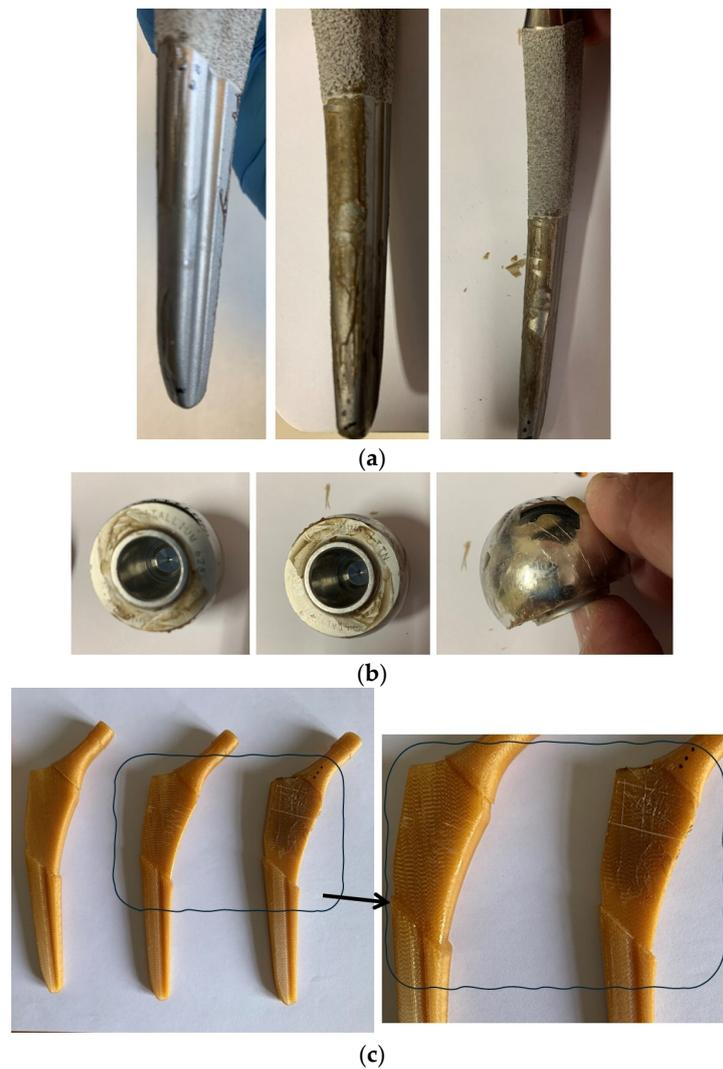
**Figure 7.** Results of adhesion tests of the biomaterial to implantable surfaces; (a) coating applied on the distal part of the Ti5 hip prosthesis; (b) coating applied to the femoral head of the hip prosthesis
