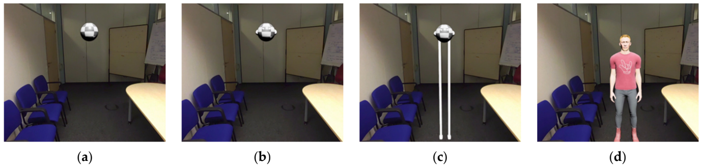
Figure 5. The projected drone models and the human male model in the room as seen through the HTC XR Elite: (a) Simple spherical form; (b) Variant with anthropomorphic features; (c) Variant with anthropomorphic features plus ground anchoring; (d) Human male model. All models are positioned with their anchor point at a height of 110% of eye level and at a distance of 2 m.
