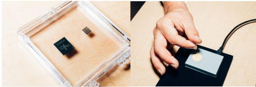
Figure 8. The challenge of Soli was to shrink the radar to the size of a computer chip. Peter Mccollough for Wired.
