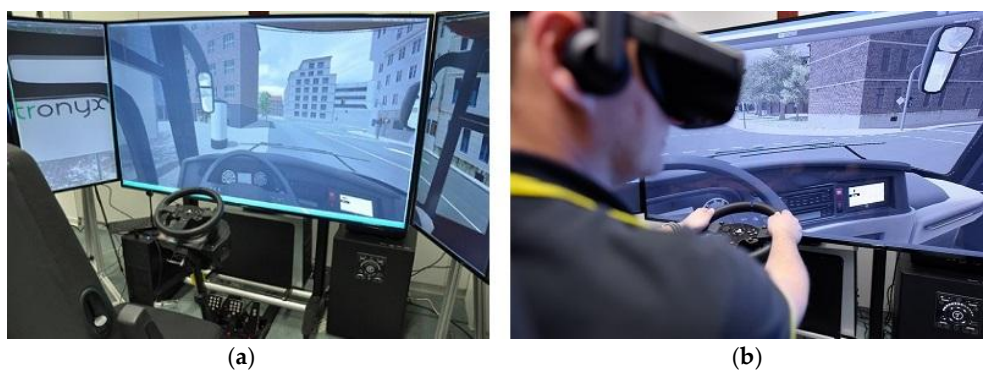
Figure 2. A driving simulator developed within the project inTraSim: (a) The hardware equipment of the developed driving simulator; (b) A test driver performing a turn-right maneuver.
