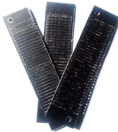
**Figure 3.** Three-layer bipolar plate (cathode side).
