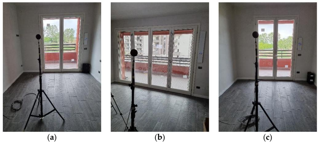
**Figure 2.** Sound pressure level measurements: (a) bedroom 1 with CM CMV, (b) living room with SM CMV and (c) bedroom 2 with CM CMV.
